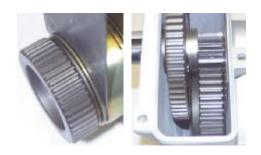
Now insert the drum retention plate. Please take care that the plate locates in the correct groove as shown opposite.
