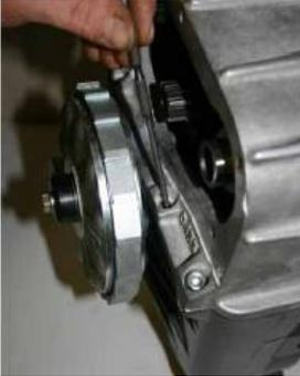
Using the scribe, mark the position of the new mounting on the lower housing, using the top housing as a guide.
