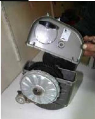
Using the ¼” Alley key, remove the 3 bolts that secure the upper motor housing & place to one side.
