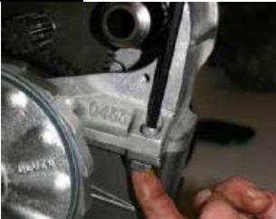
Without using sealant fit the new top housing to the winch taking care to make sure it locates correctly.
