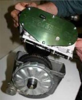
Apply a bead of silicone type sealant to the top housing and fit the winch taking care to ensure the correct location and meshing is achieved.
