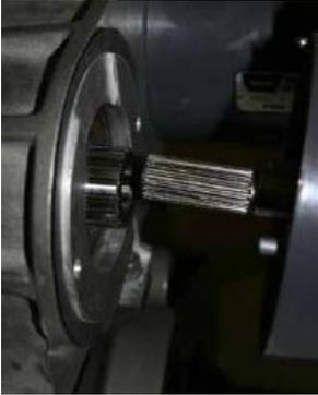
The motors can now be fitted. We recommend the use of a gasket or a small bead of silicone type sealant. We also suggest a smear of grease (Multipurpose) is applied to the shaft of the motor before engaging to the top housing.
