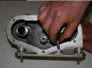
Insert the 3 bolts onto the housing as shown.
