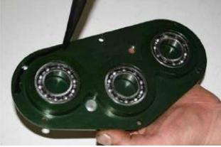
Fit the side plate to the housing using the gasket supplied. If this gasket becomes damaged for any reason, high temp silicone sealant can be used as a temporary alternative.
