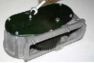
Fit the breather elbow to the housing side cover. (Recommended.)
