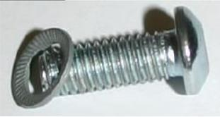
Before fitting the bolts take care that the special washers are fitted correctly with the raised inner facing the bolt head.
