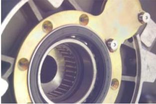
Prepare bearing retention plate and drum oil seal ready to fit. Apply anti corrosion compound to counter sunk bolt holes & align gasket. Fit and tighten all bolts evenly.
