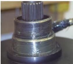
Liberal apply all purpose grease to bearing and seal surfaces on drum using a small brush.
