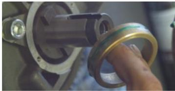
Once the mainshaft, cam gears & 48 tooth intermediate gears are in place, lay the gearbox casing down to fit the bronze bush. Ensure that the grub screw is wound out before tapping in the bush, and then gently tighten the grub screw once fitted.
