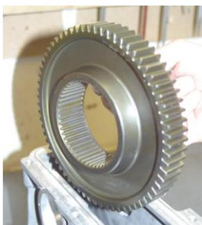
Place the large 50 tooth gear into the lower housing with the shoulder facing towards the smaller hole.
