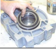
Degrease bearing aperture & bearing. Apply sealant & fit. Knock home carefully with a soft blow hammer.
