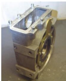
Remove winch drum & strip winch completely so that lower housing is bare.
