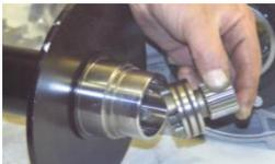
Apply silicone grease to "o" ring seals on piston gear, align with drum and push into place.
