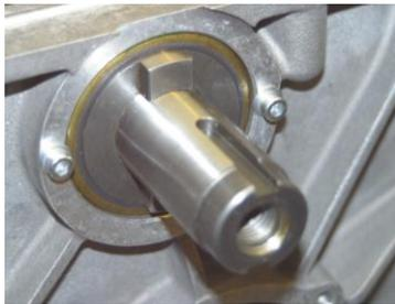
Now fit the gearbox housing oil seal & tighten the retaining bolts..
