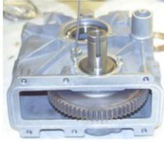
Insert the mainshaft & cam gears into the gearbox and through the intermediate gear, make sure the mainshaft & smaller cam gear pass through the spacing washer & circlip. The mainshaft must be fully seated into the support bearing! Now fit the large circlip to the small cam gear.
