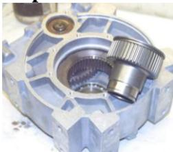
Turn the housing over and fit the large gear into the 50 tooth main gear. Take care not to damage the bearing on the other side of the casing.
