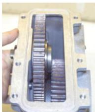
Fit 48 tooth intermediate gear into lower housing with the shoulder facing the large hole. Ensure that the large spacing washer & circlip are to hand ready for step 5.
