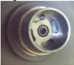
Prepare winch drum ready to fit. Apply rubber grease to "o" ring seals on drum insert. Ensure drum insert is aligned, then push into place. Apply thread lock compound to securing bolt and tighten.
