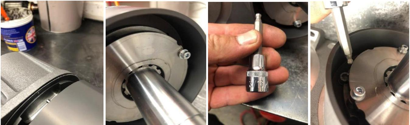
The next step is to install the end cap, with the air fitting on the top, fit the 4 x M6 cap head bolts and schnoor washers, using a little copper slip on the threads, tighten with a 5mm allen key.
