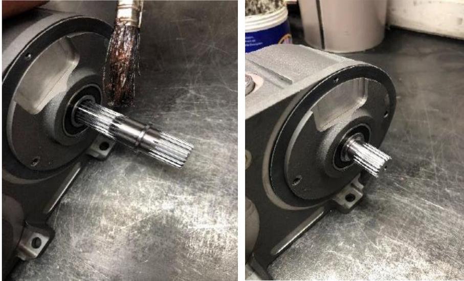
Slide the gear shaft onto the installed drive shaft, with the gear teeth closest to the top housing.
